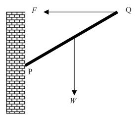
Which of the following diagrams best shows the correct direction of the reaction force R at the hinge?
