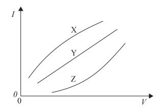
Which of the following corresponds to resistors for which the resistance increases with increasing current?
