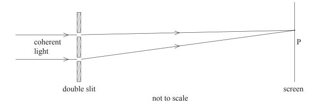
The light from the two slits has equal amplitudes on reaching point P.
