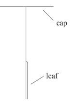
A positively charged rod is brought near to the cap of the electroscope.
