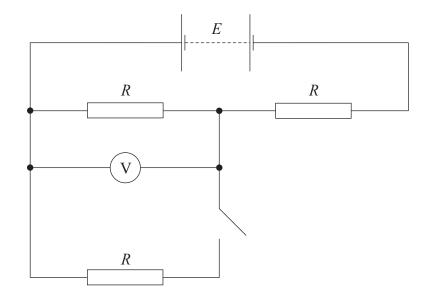
The voltmeter has infinite resistance.
