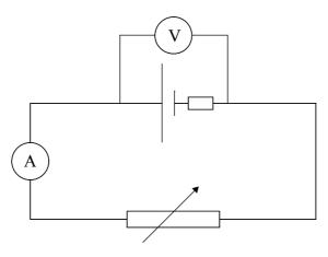
correct position of voltmeter; correct position of ammeter; correct position of variable resistor;
