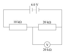
The reading on the voltmeter is
