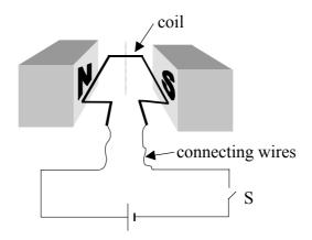
With the coil in the position shown, when the switch S is closed the coil will
