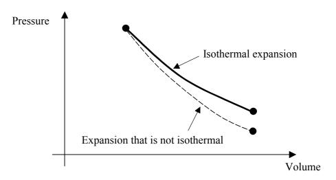
In the expansion that is not isothermal, the internal energy of the gas
