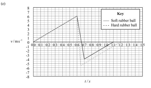
$0 \rightarrow 0.6$  s is the same; shorter contact time; speed greater leaving floor; same slope for rebound; longer time to reach max rebound height;
