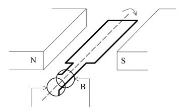
At the instant when the rotating coil is oriented as shown, the output emf of the generator
