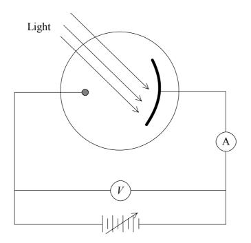
If the intensity of the incident light is gradually increased, the stopping potential required will
