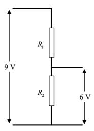
The ratio of the resistances  $R_1$ :  $R_2$  must be
