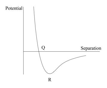
Which feature of the curve best helps explain the phenomenon of the expansion of the solid with increasing temperature?
