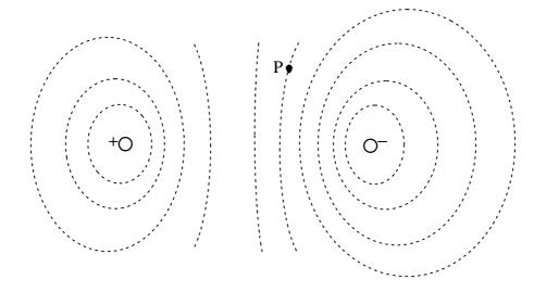
**28.** The diagram below shows equipotential lines in the vicinity of two unequal charges.
