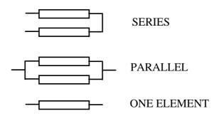
Which line in the table below indicates the way the heating elements must be connected to a power supply in order to provide the three settings?
