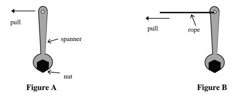
The torque exerted on the nut in Figure B compared to that in Figure A
