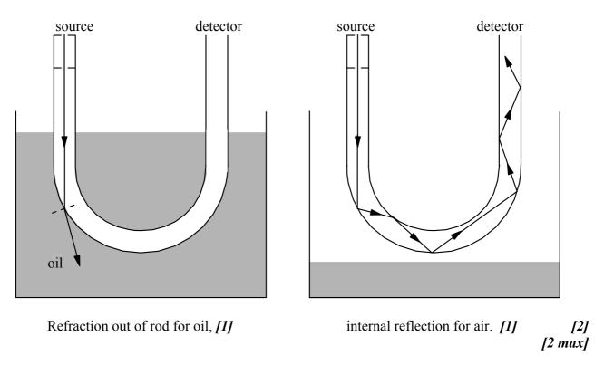
(Note: there is a small reflected ray in addition to the refracted ray for the diagram on the left, but do not require it.)
