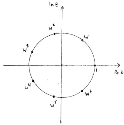
7 points equidistant from the origin approximately correct angular positions for  $1, w, w^2, w^3, w^4, w^5$  and  $w^6$
