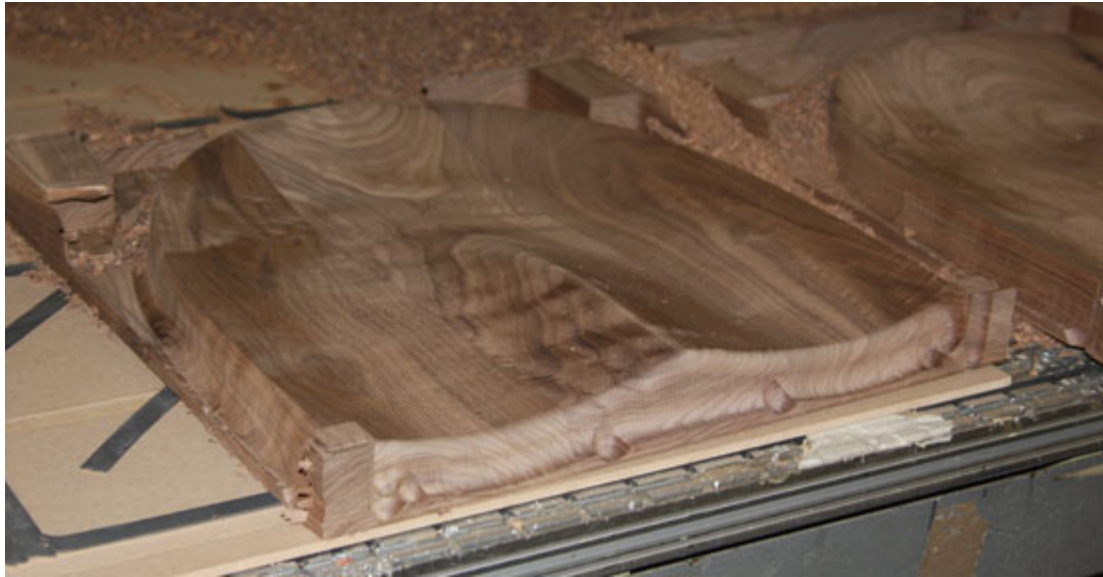
Figure C3: A chair seat made from hardwood using a CNC router
