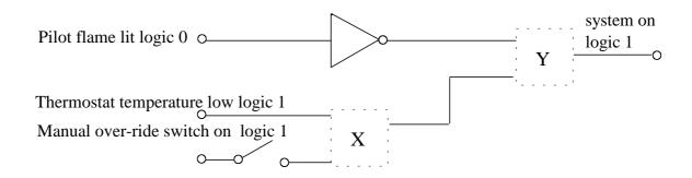
**28.** Which logic gates should be placed at X and Y in the circuit so that the system turns on if the pilot light is on and the thermostat temperature is low or the manual over-ride switch is on?
