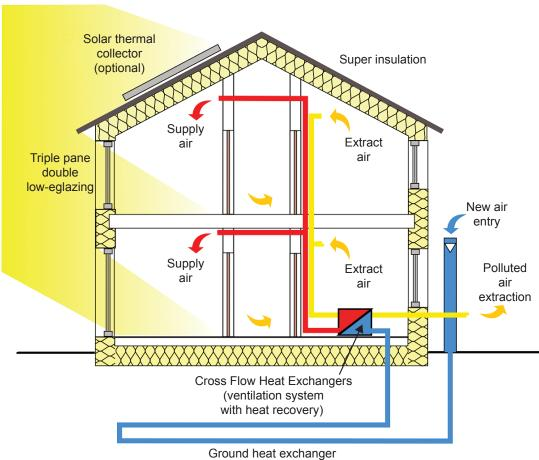
Figure 8: The Passivhaus
