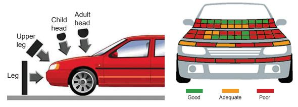
Figure 10: Testing cars for pedestrian protection
