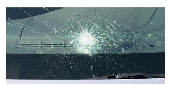
Figure 6: A car windscreen damaged by impact
