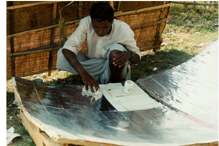
Figure 5c: A parabolic solar cooker produced in Nepal from local materials
