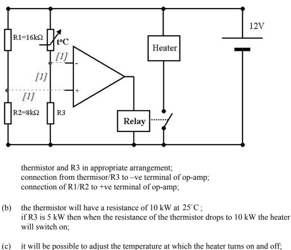
(c) It will be possible to adjust the temperature at which the heater turns on and off; by adjusting the variable resistor; [2 max]
