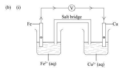
correct diagram including voltmeter/meter, 4 correct species (state symbols not required) and connecting wires;
