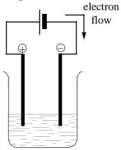
Labels are not required. one container, two electrodes, battery (and electrolyte);
