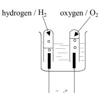
*Or similar suitable diagram.* gas collection method; names of gases correct way round at electrodes; 2:1 volume ratio correct way round; [3] (i) mass increases; copper deposited; because X is negative and attracts  $Cu^{2+}$  ions / reduction occurs at X / [3]  $Cu^{2+} + 2e^{-} \rightarrow Cu;$
