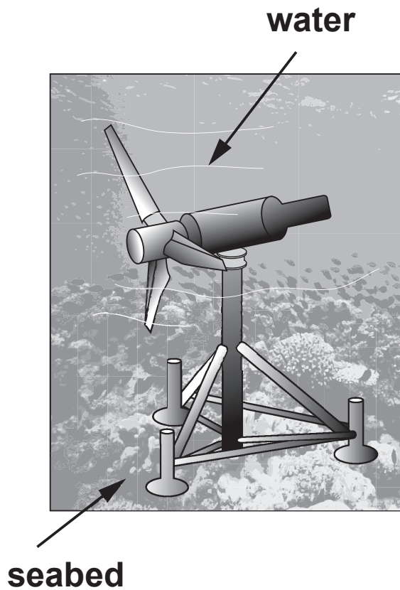
tidal water turbine
