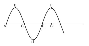
The distance between point ..... and point ..... is equal to one wavelength.
