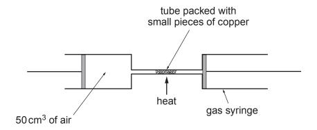
50 cm³ of air was trapped in one of the syringes. The air was passed forwards and backwards over the heated copper. The copper reacted with the oxygen in the air producing solid copper(II) oxide. The final volume of gas was recorded when the apparatus had cooled to room temperature.
