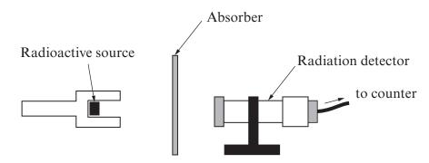
A number of different absorbers are placed, one at a time, between the detector and the radioactive source.
