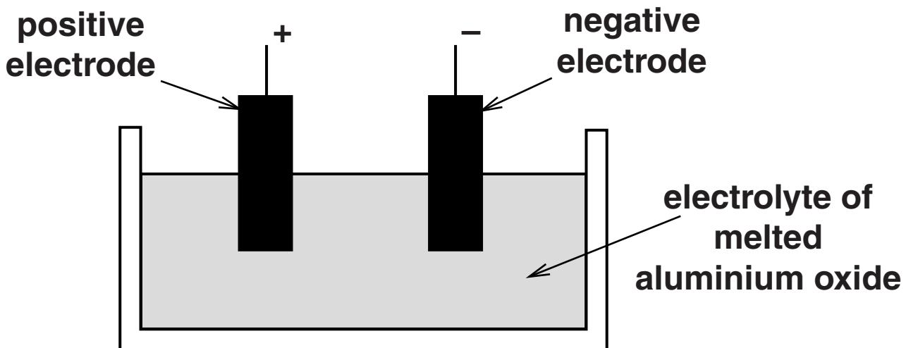
**The aluminium oxide,  $\text{Al}_2\text{O}_3$ , breaks down into aluminium and oxygen.**
