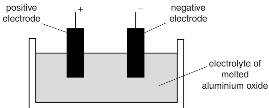
The aluminium oxide,  $\text{Al}_2\text{O}_3$ , breaks down into aluminium and oxygen.
