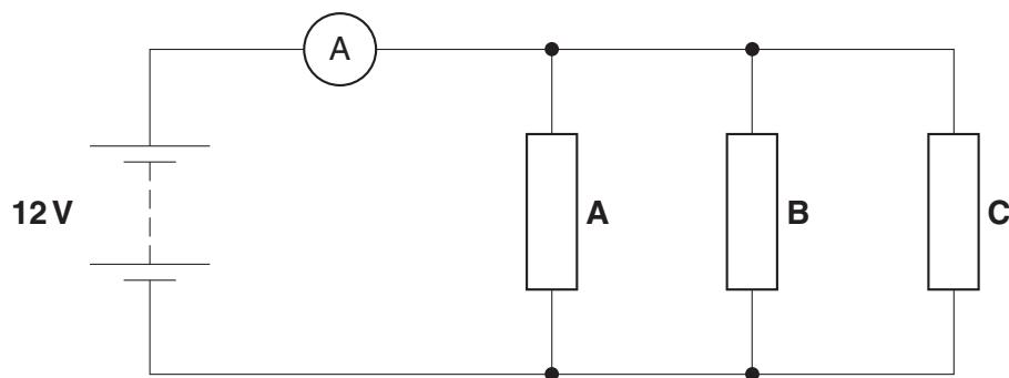
The ammeter in the circuit reads 6A.
