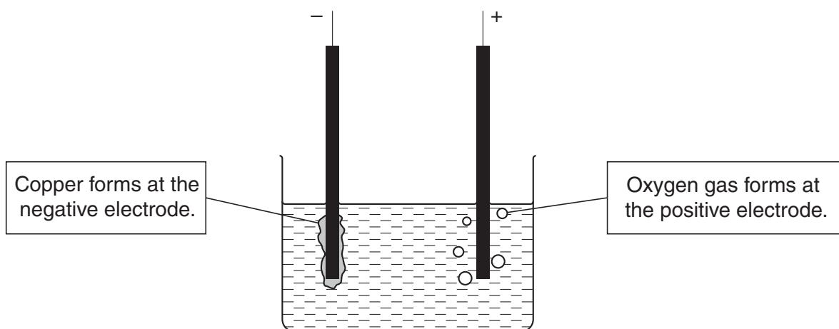
During the electrolysis process, copper ions ( $\text{Cu}^{2+}$ ) change to copper atoms.
