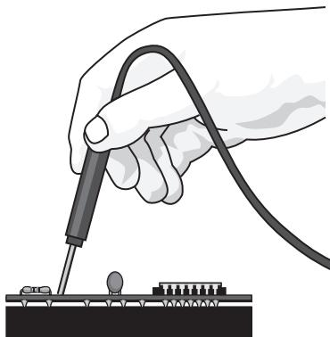
He needs to be careful. The chips in the circuit are easily damaged by static electricity.
