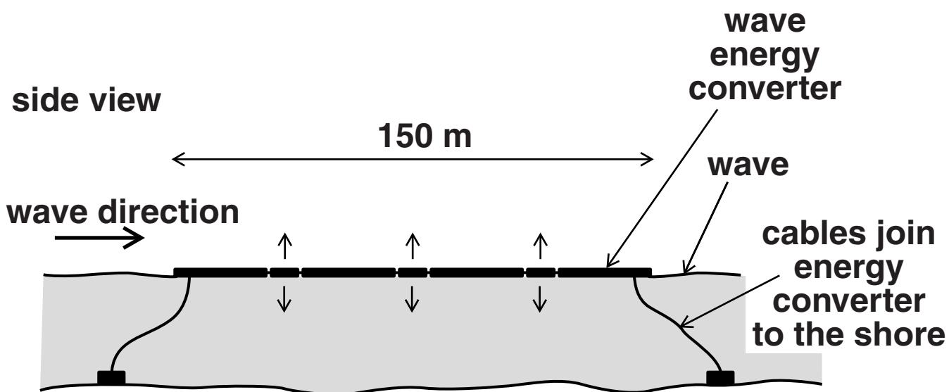
**As the wave passes, the wave energy converter bends at its three joints. This pumps oil through hydraulic motors, which then drive generators. The electricity they produce passes along cables to the shore.**
