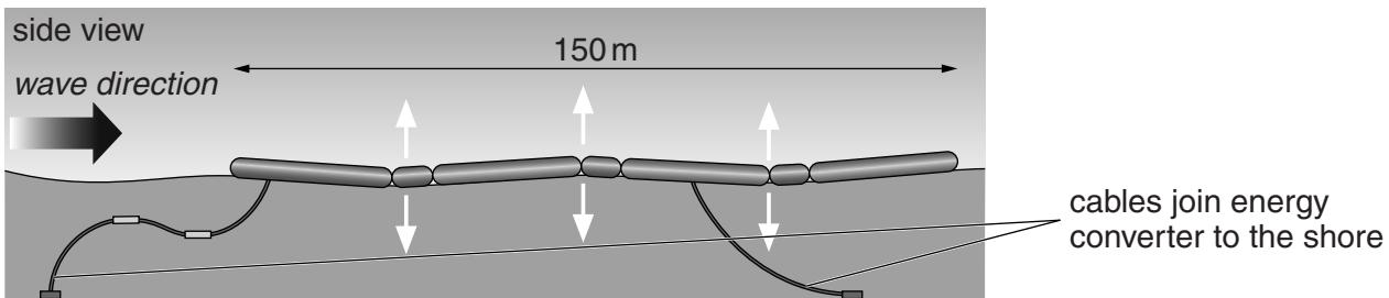
As the wave passes, the wave energy converter bends at its three joints. This pumps oil through hydraulic motors, which then drive generators. The electricity they produce passes along cables to the shore.
