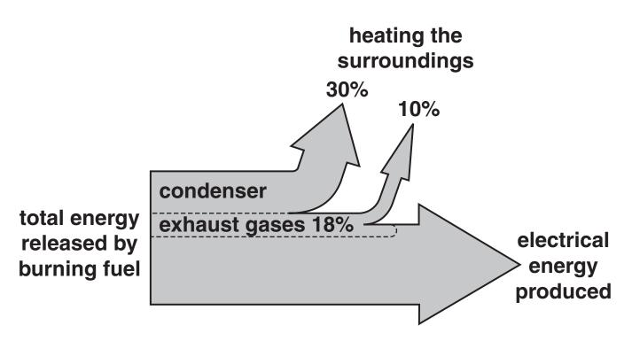
(ii) The diagram shows the efficiency of this power station.
