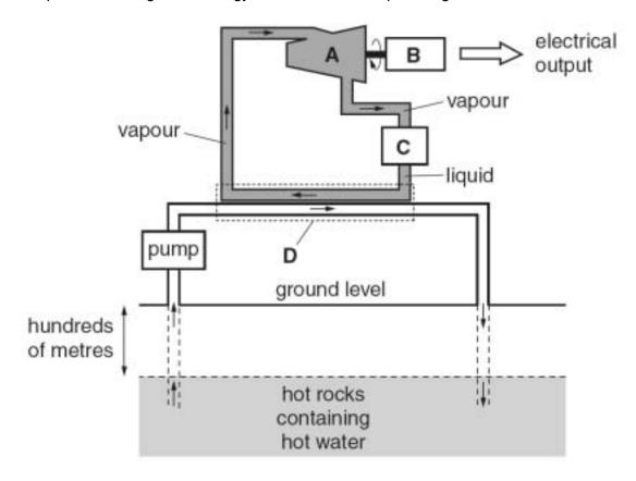
The four parts labelled **A**, **B**, **C** and **D** in the diagram are a condenser, a generator, a heat exchanger and a turbine.
