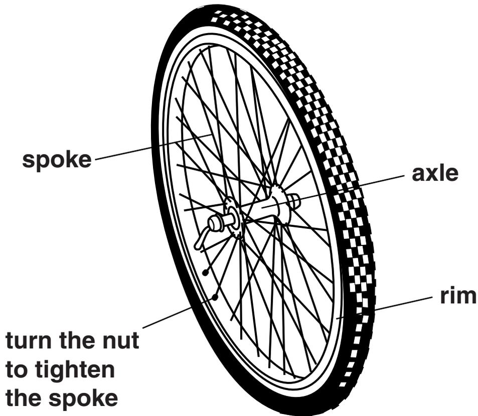
**He clamps the axle firmly and uses a force to make the rim bend (deflect) sideways.**
