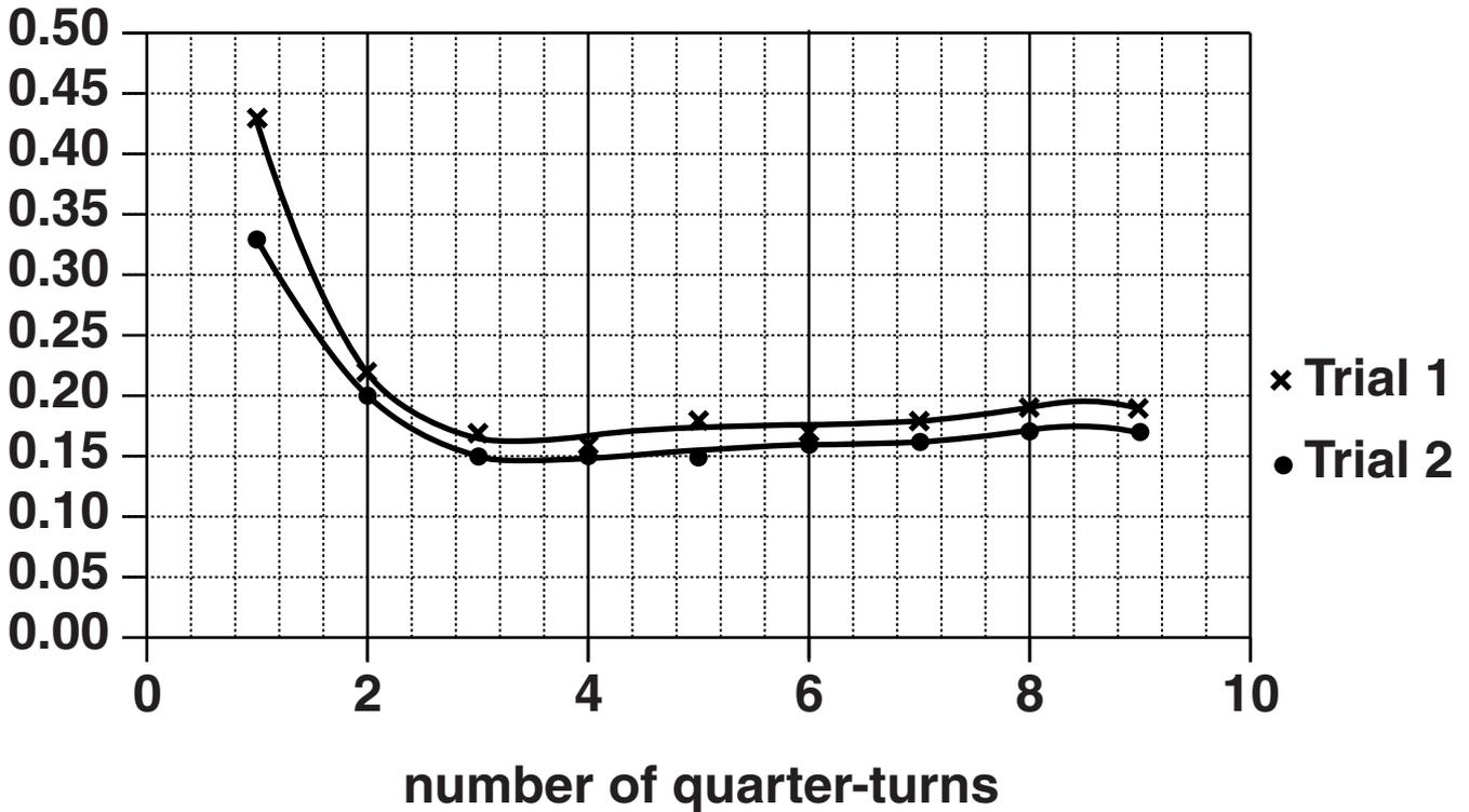
The graph shows that the wheel is flexible if the spokes are loose and stiff if the spokes are tight.
