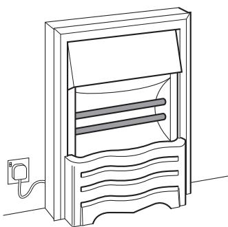
The bars in the heater are resistors.
