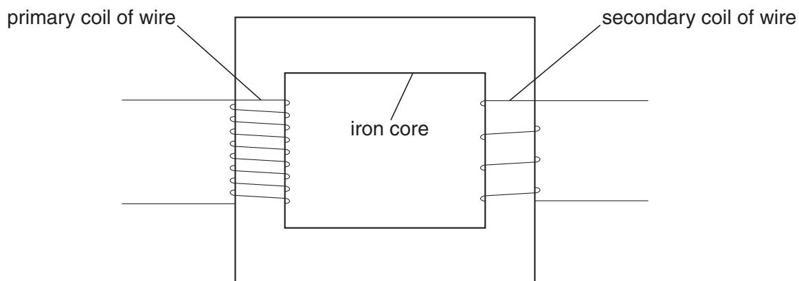
Explain how a transformer produces a voltage across the secondary coil.
