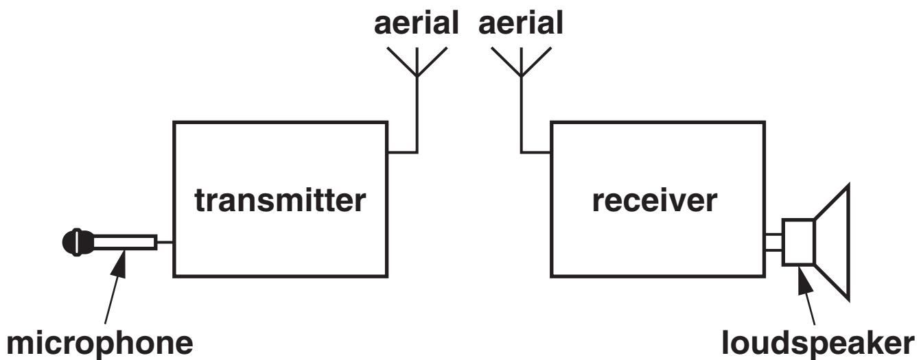
**The microphone collects the analogue sound signals, which are then converted into digital radio signals. The digital radio signals are sent to a receiver.**
