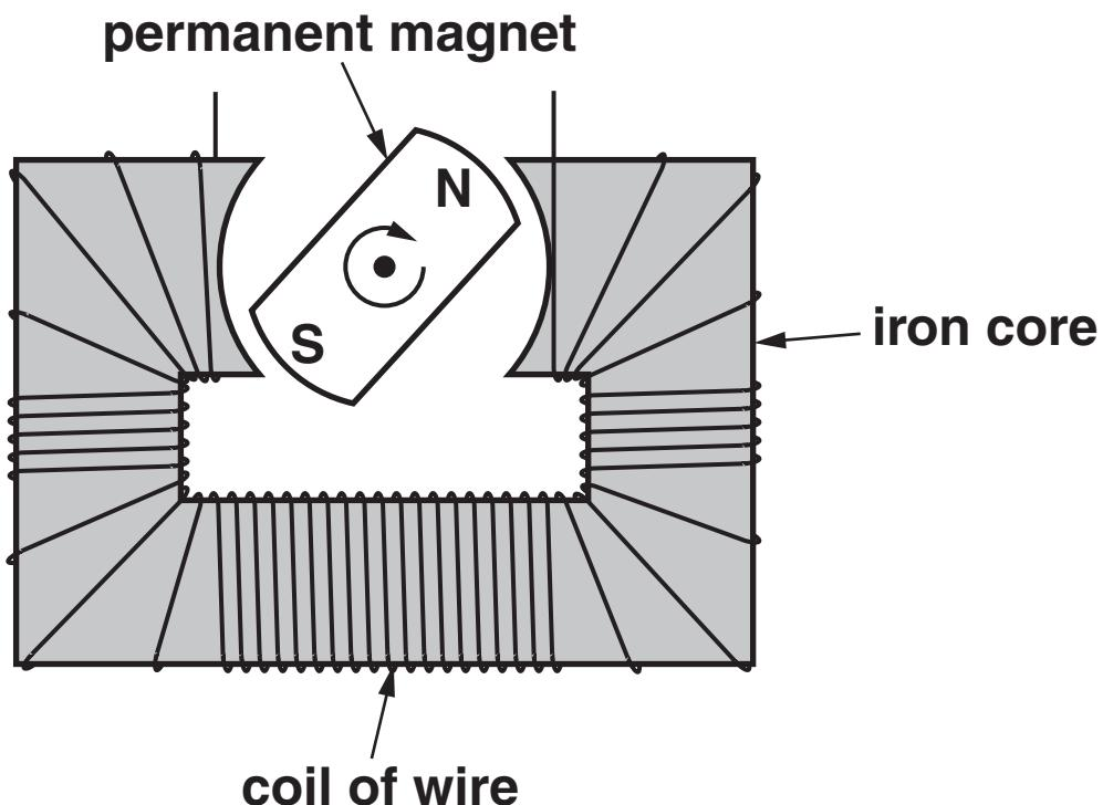
**Describe how a simple generator produces electricity.**
