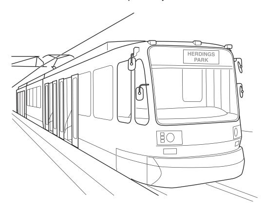
The supertram is 34.8 m long and 2.65 m wide. This makes it one of the largest articulated cars ever built for public transport. An empty supertram has a mass of about 50000 kg. It can carry 88 people sitting down and an extra 162 passengers standing. The supertram has a top speed of 80 km/h. There is an enormous change in momentum when the supertram pulls away from a stop and reaches top speed.
