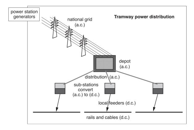
The supertrams run on a 750 volt electrical supply. They use electricity from the national grid. This is transmitted as an alternating current (a.c.). The a.c. electricity is produced by generators in the power stations. The electricity is distributed across the tramway network as a.c. At local sub-stations near the rails it is transformed to the correct voltage for the overhead cable (750 volts) and converted to a direct current (d.c.).
