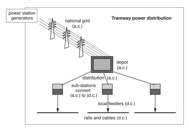
The supertrams run on a 750 volt electrical supply. They use electricity from the national grid. This is transmitted as an alternating current (a.c.). The a.c. electricity is produced by generators in the power stations. The electricity is distributed across the tramway network as a.c. At local sub-stations near the rails it is transformed to the correct voltage for the overhead cable (750 volts) and converted to a direct current (d.c.).
