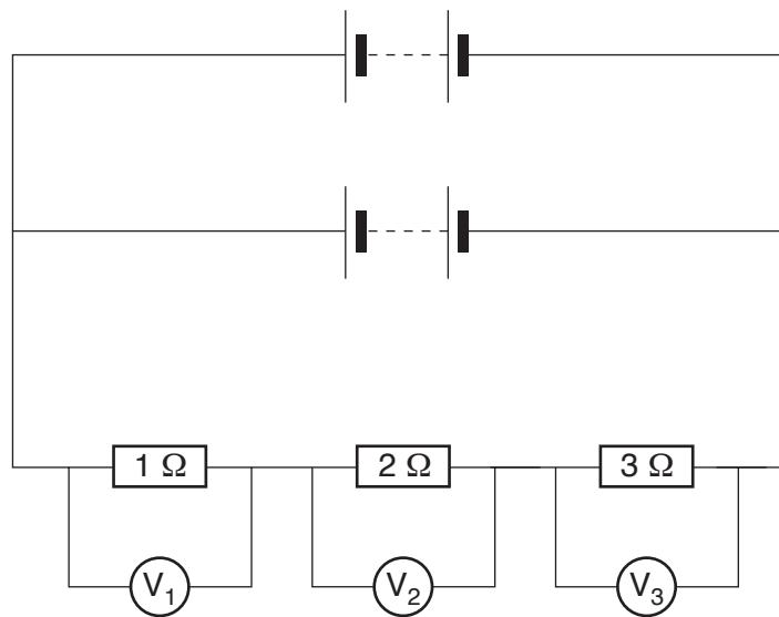
What effect will the additional battery have on the voltage across the resistors?
