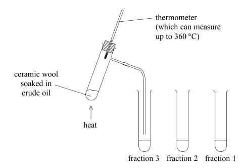
The table gives information about four fractions that were separated using this apparatus.
