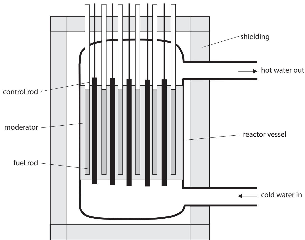
Chain reactions in the reactor release energy.
