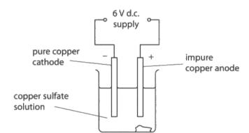
The electrolysis was carried out for a period of time. The electrodes were removed, washed, dried and their masses redetermined.
