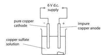
The electrolysis was carried out for a period of time. The electrodes were removed, washed, dried and their masses redetermined.
