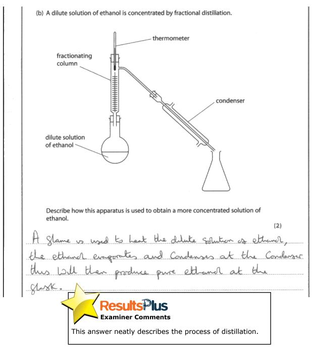
(b) A dilute solution of ethanol is concentrated by fractional distillation.
