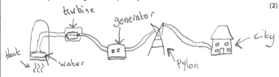
the heat from a nuclear reactor heats water and forms Steam. The Steam then rises and turns a turbine as the turbine Spins electrical energy will be produced in a generator and get transcried to the Pylons and then to a city (Total for Question 2 = 8 marks)
