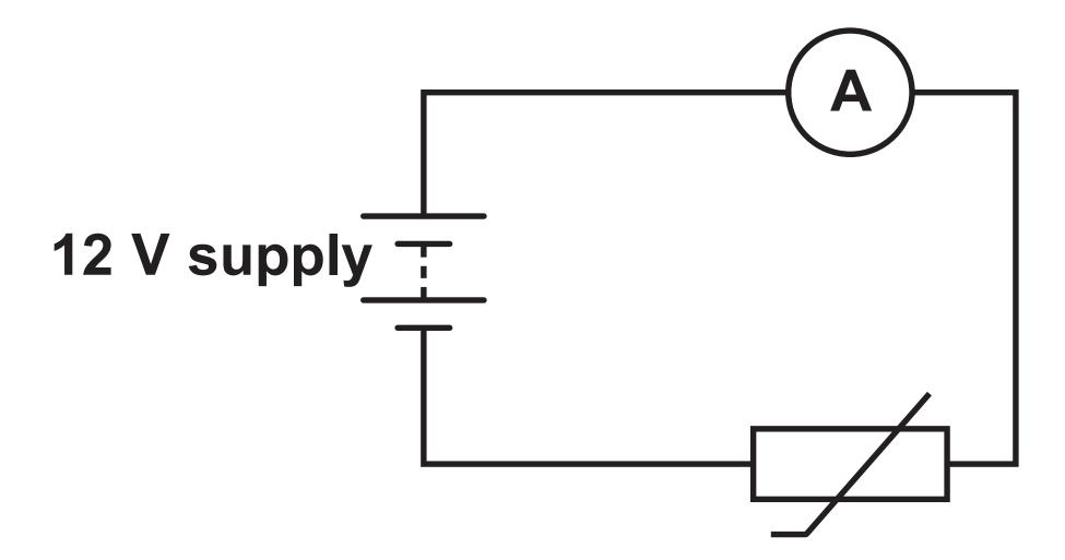
He heats the thermistor and measures the current at different temperatures. On page 19 are some of the results plotted on a graph.
