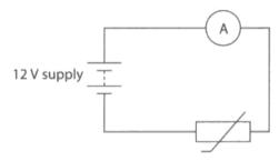
He heats the thermistor and measures the current at different temperatures. Here are some of the results plotted on a graph.
