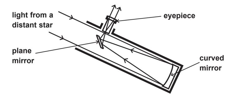
(i) Describe what the mirrors and the eyepiece do to the light rays to form an image of a distant star. (3 marks)
