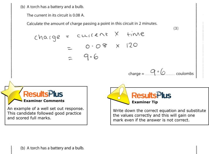
The current in its circuit is 0.08 A. Calculate the amount of charge passing a point in this circuit in 2 minutes. Charge = Current x time (3)  $0.08 \times 2 = 0.16$  charge = 0.16 coulombs Charge = 0.16 coulombs Charge = 0.16 coulombs (b) A torch has a battery and a bulb.
