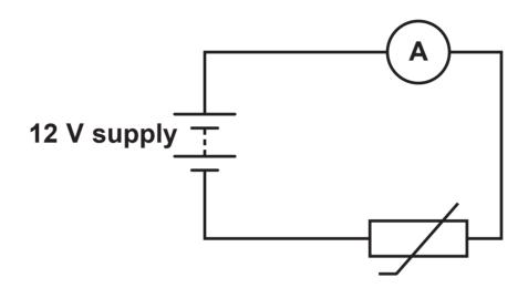
He heats the thermistor and measures the current at different temperatures. On page 15 are some of the results plotted on a graph.
